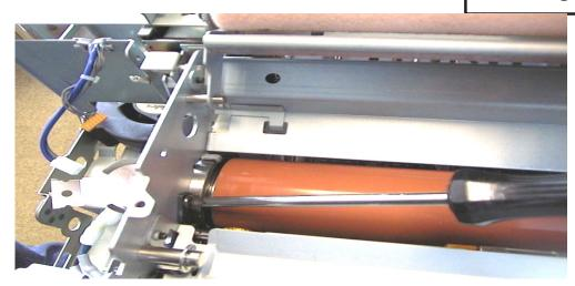
With a screwdriver fitted to the screw (XB1-2400-807), attach the nut (XB7-2100-409) then tighten it. While doing this prevent the screw from turning by holding the screwdriver stationary.
