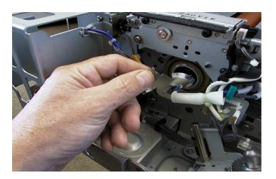
Remove the fixing cleaner belt drive assembly (two screws), this exposes the screw that holds the reciprocating shaft bushing in place.
