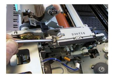
• Remove heater cover plate from the front of the upper fixing roller, as shown.
